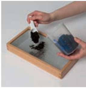
1a) Using sieves to homogenize the soil sample
