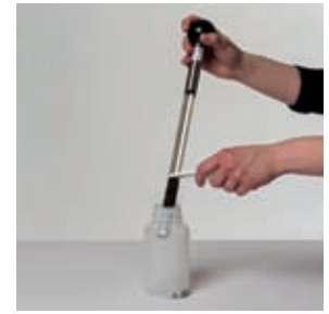
1c) Measuring the sample volume using the graduated sampling auger (e.g. for mineral soils)
