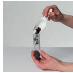
1b) Measuring the sample volume with the graduated sample container (e.g. for horticulture gardening substrata)
