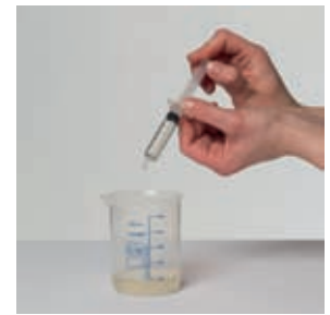
5) Measuring the filtrate with a graduated plastic syringe
