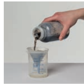
4) Filtration of the extract using a round filter
