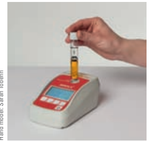
9) Insert the cuvette into the AMOLA® base unit. Read the measured value directly in kg/ha (mineral soils) or mg/l of substrate (for substrates), or ...
