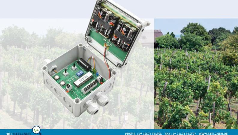
Extra features include an additional relay with potential-free switching for AC solenoid valves, an additional release option with thermostat or external float switch, as well as the forwarding of the measured values as analogue signals.
